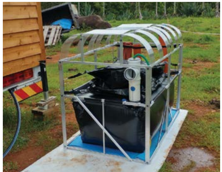
Biogas digester. Image credit: Living Tiny and Green
